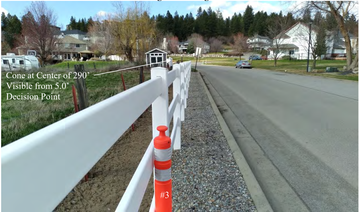
Photo 9 – From 5.0' Decision Point looking north for right turn movement
